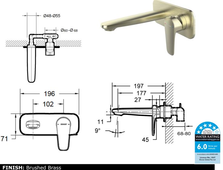
**CONSTRUCTION:** Super Brass **CARTRIDGE: 35mm Ceramic** CONNECTION: 1/2Ø BSP Female WORKING PRESSURES: 150 - 500 Kpa **OPERATING TEMPERATURE:** 5°C - 70°C WELS RATING: 5 Star - 6.0L/m Warranty: 15 Years Warranty & Lifetime on cartridge\* (Terms & Conditions Apply)
